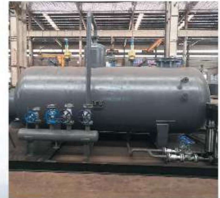
Thermal oil steam generator in Egypt
